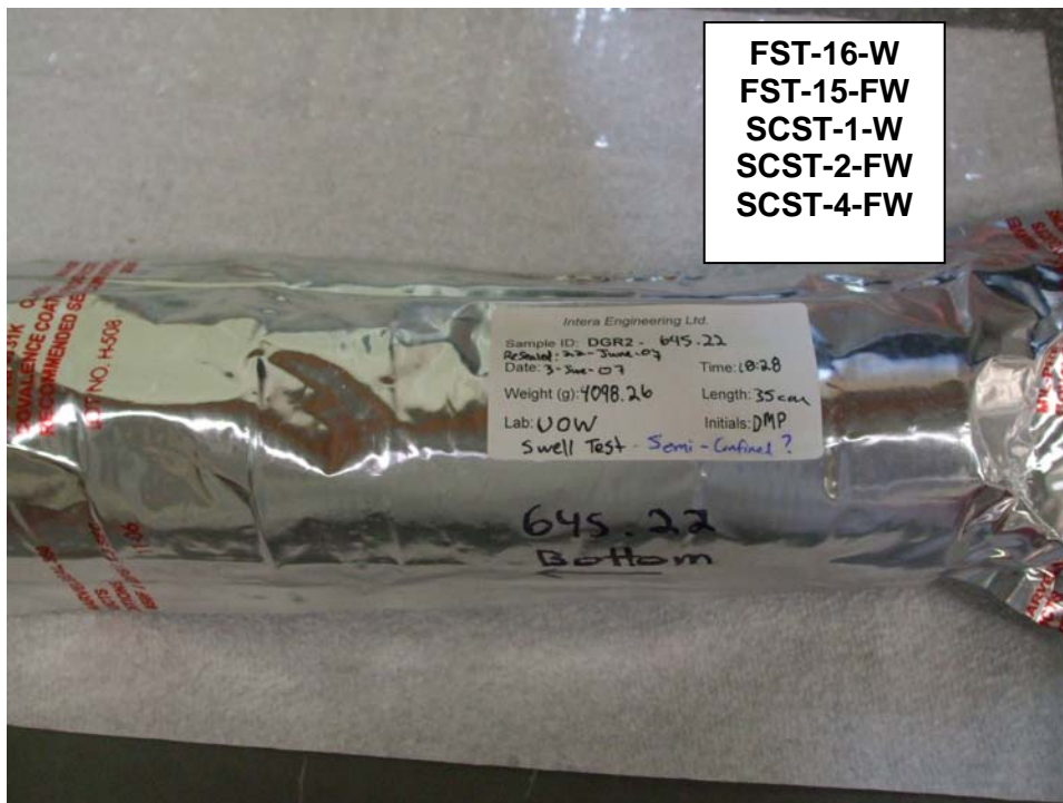
Figure A4 (b). Blue Mountain Formation – Sample DGR2-645.22 (Received on June 26, 2007); Sample broken designated for Semi-confined swell tests
