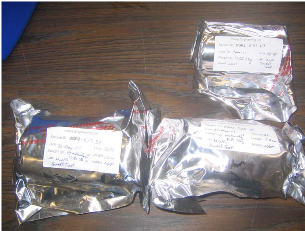
Figure A1. Cores Received in Double Vacuum-sealed Polyethylene and Aluminum Foil Bags
